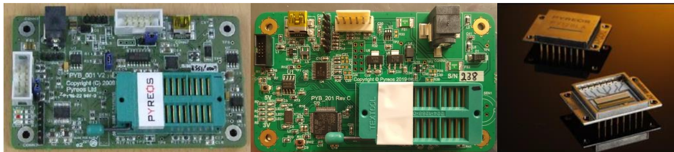
Figure 1: Linear Array Evaluation Kit contents (Evaluation board variations PYB_001 V2 and PYB_201 Rev C, and the linear array sensor)
