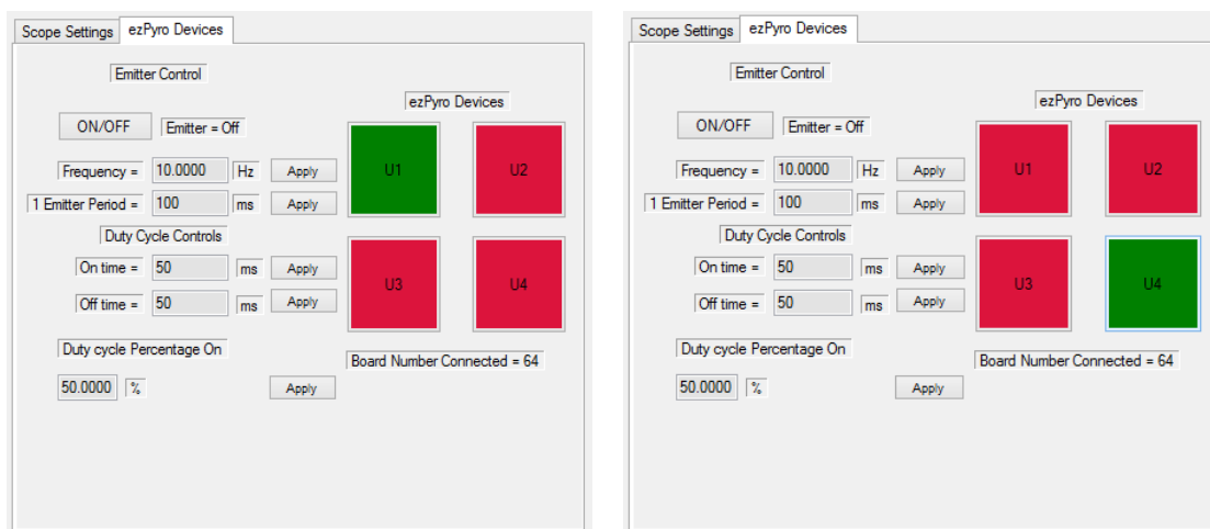
Figure 24: ezPyro™ Devices tab in Single Device programming mode with U1 (left) and U4 (right) settings selected
